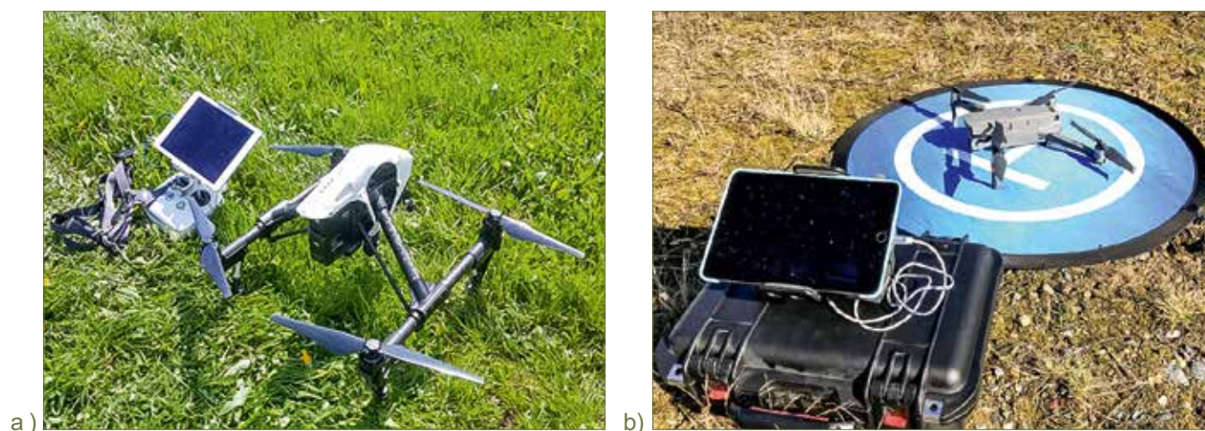
Fig. 1: Imaging platforms, used for monitoring. a) DJI Inspire 1 Pro, b) DJI Mavic 2 Pro.
