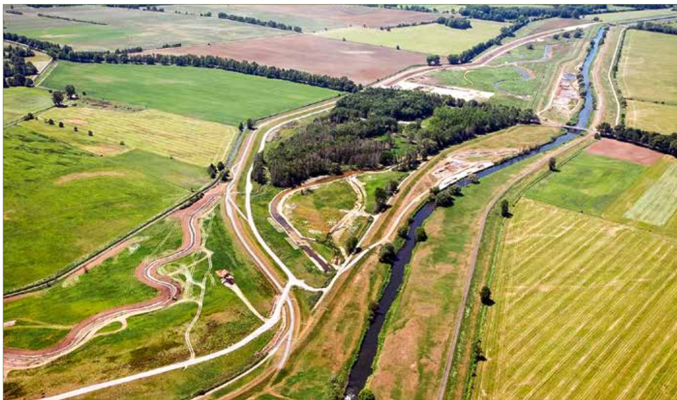
Fig. 2: The dyke was relocated up to 3 km, 45 ha of new floodplain and a new water network were created
