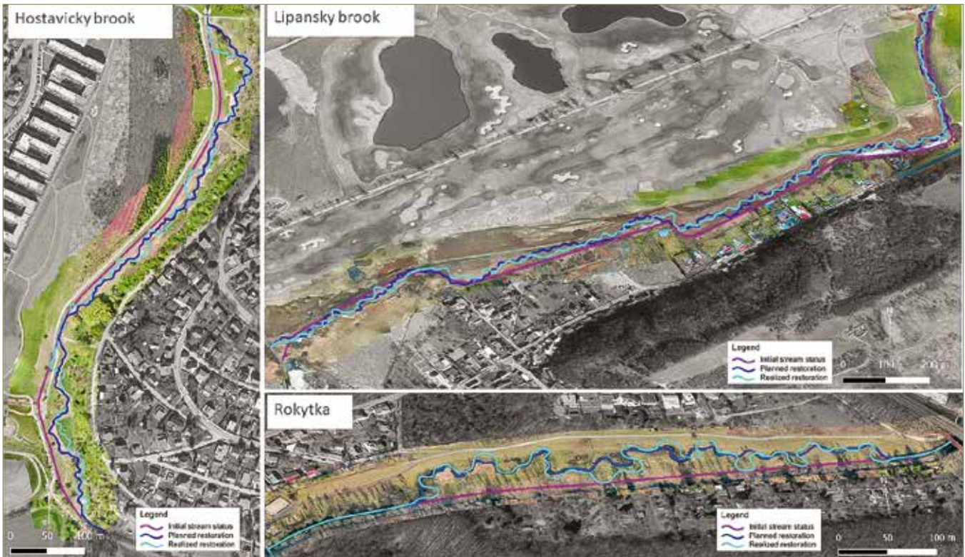
Fig. 2: Difference of the realized stream restorations to the planned and initial status.
